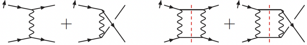
Figure 2.7: Left: Tree-level Feynman diagrams for transversely polarized electron-electron scattering, showing the basic exchange processes. Right: One-loop Feynman diagrams, contributing to the azimuthal asymmetry in transversely polarized Møller scattering. The absorptive components are highlighted by the dashed red line ( s -channel cuts). These diagrams focus solely on box contributions to observe the effects of transverse spin, which are marked by arrows on the incoming electron lines [42].
