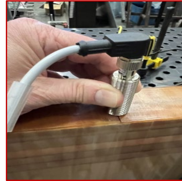
Inductance Probe measuring epoxy thickness
