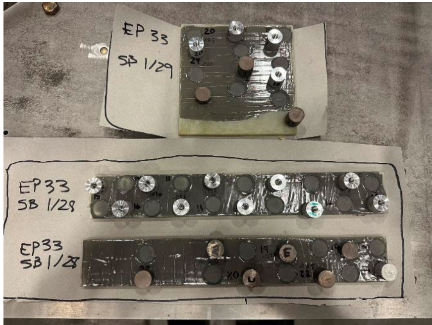
\frac{3}{4} " diameter W/Cu and Al 7075 samples post torsional shear testing
