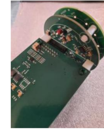
Fix the current mode amplifier with M3 screws
