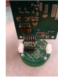
Insert the pins into the head connector
