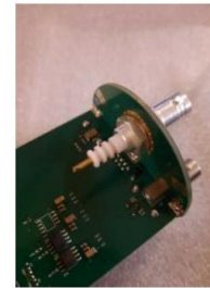
Install SHV connector
