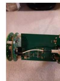
Solder HV wire
