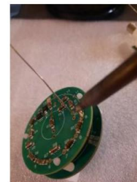
Connect the pulse mode amplifier with voltage divider using wires
