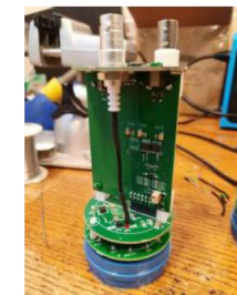
Solder PMT socket onto the voltage divider to complete the assembly
