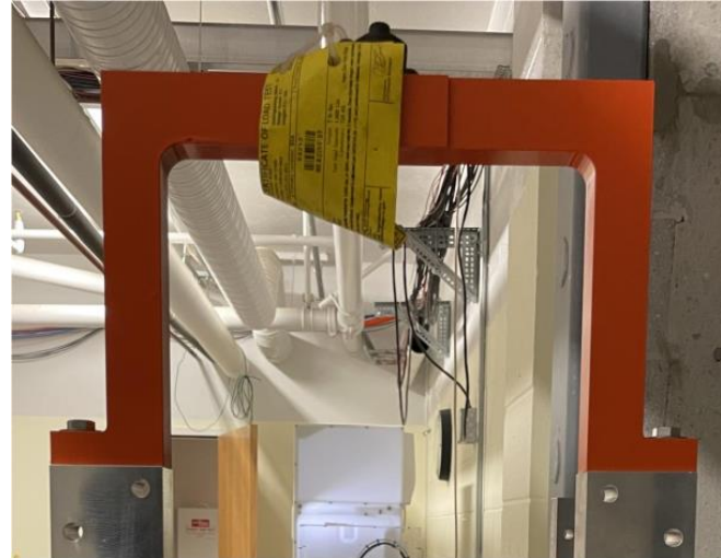
Lifting Fixture (orange painted steel)—used to mount modules to the ring
