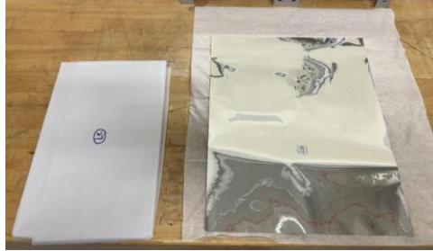
Quartz wrapped in al. mylar for protection
