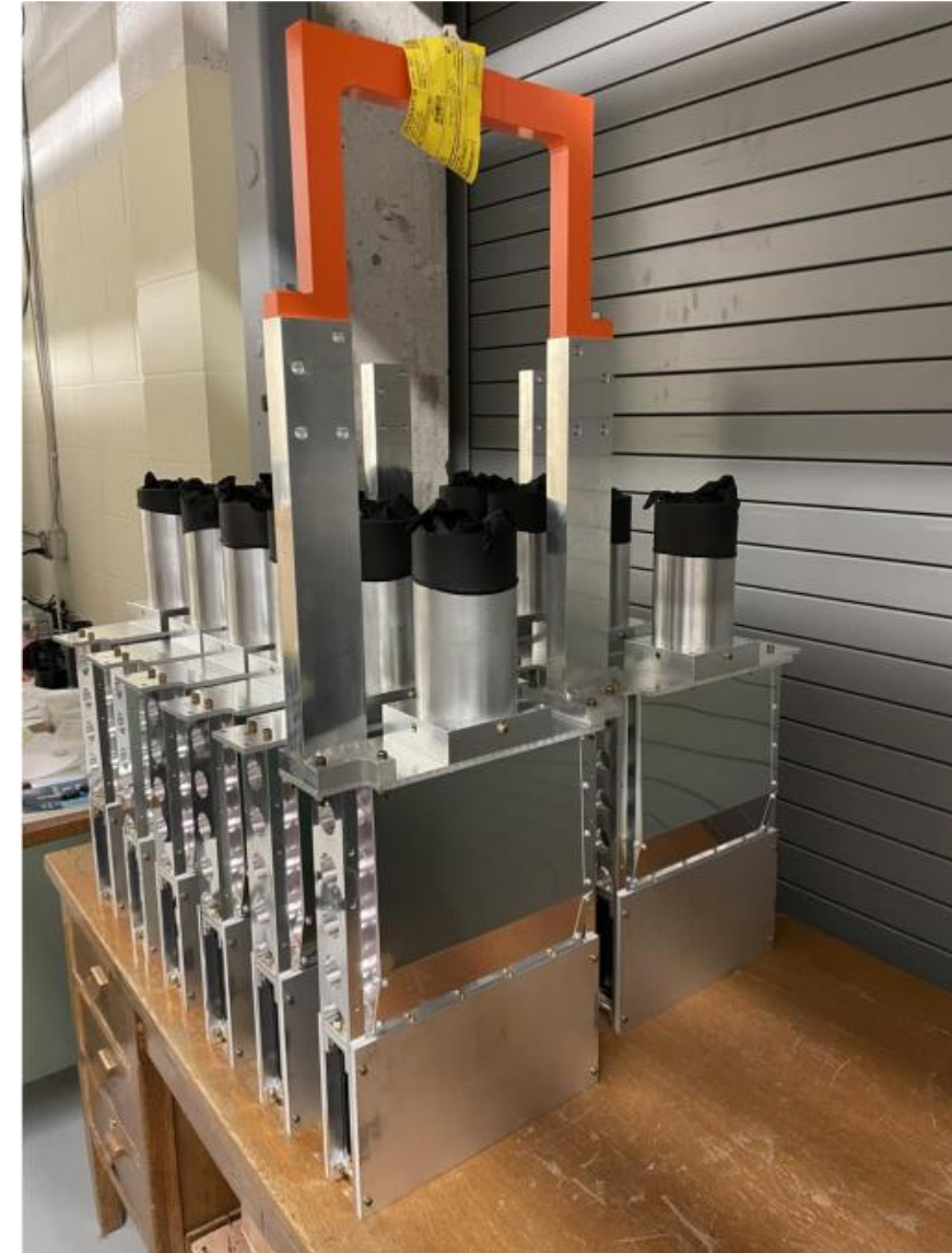
Lifting Fixture (orange painted steel)—used to mount modules to the ring
