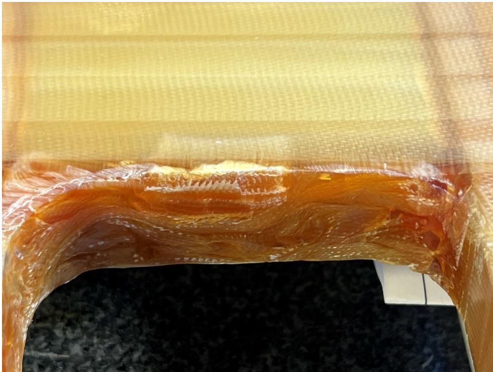
Figure 53 - Enhanced View of the Lead Side SC2-01 at Cycle 80 (End of Testing)
