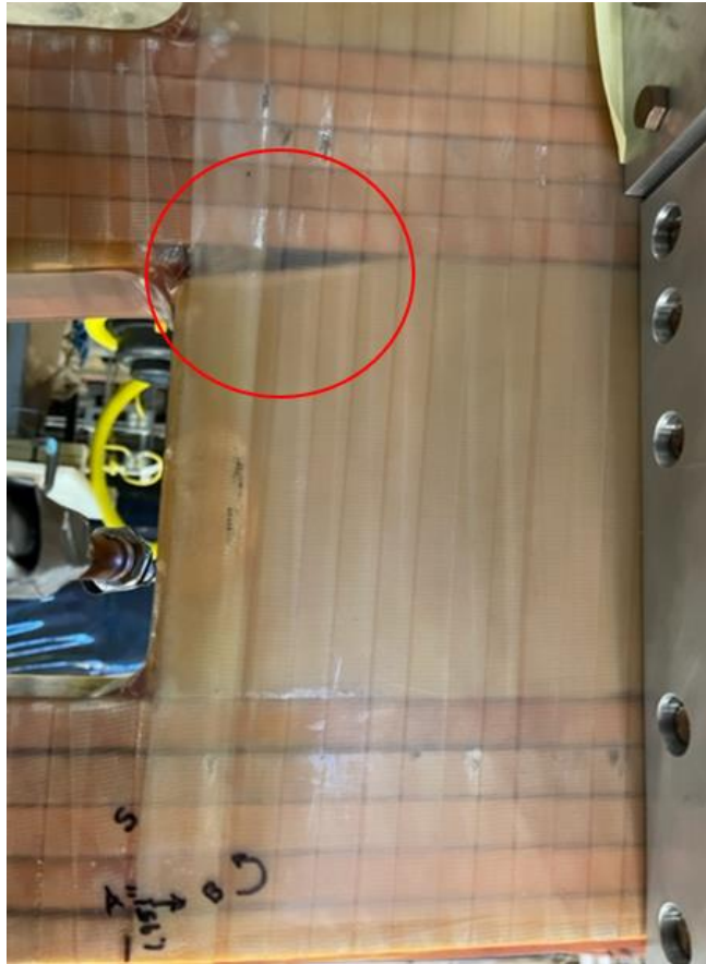
Figure 7 - Machining Error on the Inner G10 block of SC4-01, Upstream End, Right Side
