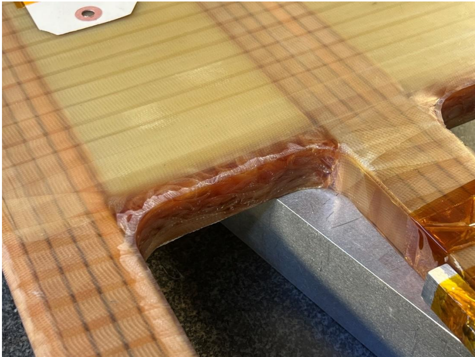
Figure 55 - Non-Lead Side of SC2-01 at Cycle 80 (End of Testing)
