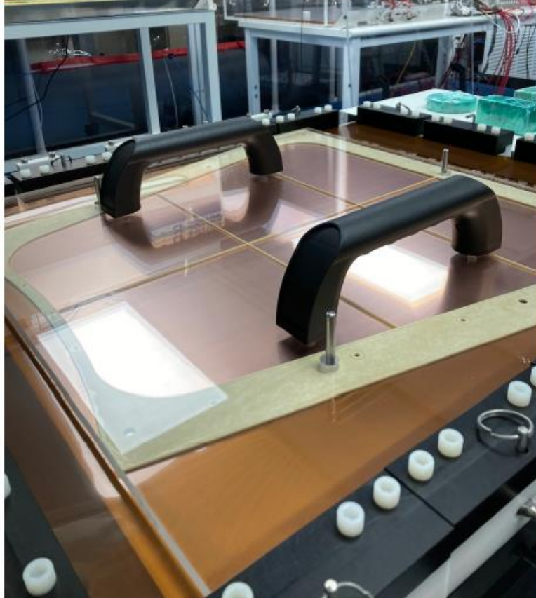
Frame on stretched GEM foil
