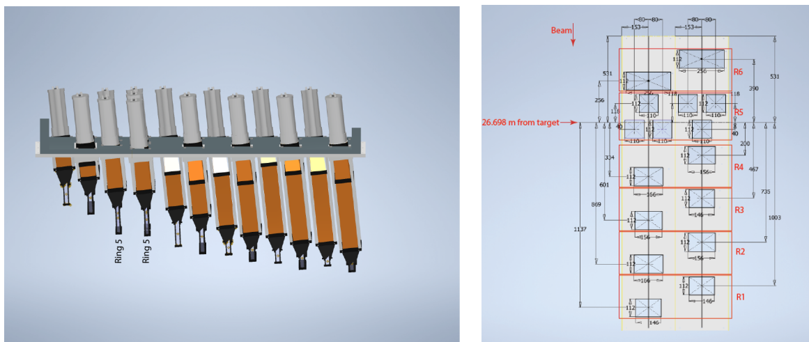
Figure 91: Left: CAD illustration of two adjacent front-flush and back-flush detector segments, illustrating the detector module positioning in the beam direction ( z -axis), with the beam traveling from left to right in the figure. Right: Front-flush and back-flush segment plates with module openings, illustrating the arrangement of the staggered detector elements.
