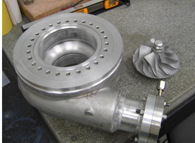
Figure 33: The LH2 pump volute and impeller.
