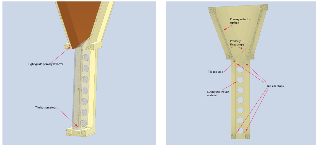
Figure 121: Cutaway view of the lower part of the quartz-light-guide tray, showing the quartz tile mounting concept and the location of the primary mirror with respect to the quartz tile.
