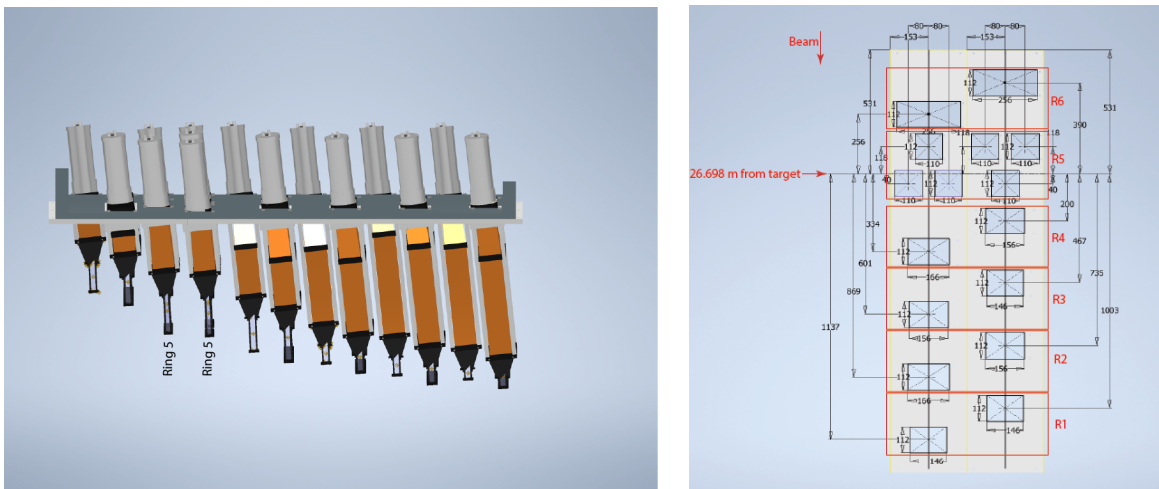
Figure 90: Left: CAD illustration of two adjacent front-flush and back-flush detector segments, illustrating the detector module positioning in the beam direction ( z -axis), with the beam traveling from left to right in the figure. Right: Front-flush and back-flush segment plates with module openings, illustrating the arrangement of the staggered detector elements.
