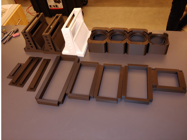
Figure 122: 3D printed parts of the detector modules for Rings 1, 2, and 5. The white tray part consists of SLS (selective laser sintering) printed nylon-12 parts, while the black pieces are Onyx (carbon fiber filled nylon) 3D printed parts.
