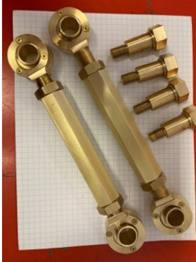
Figure 62: Brass struts for use in the US torus enclosure.
