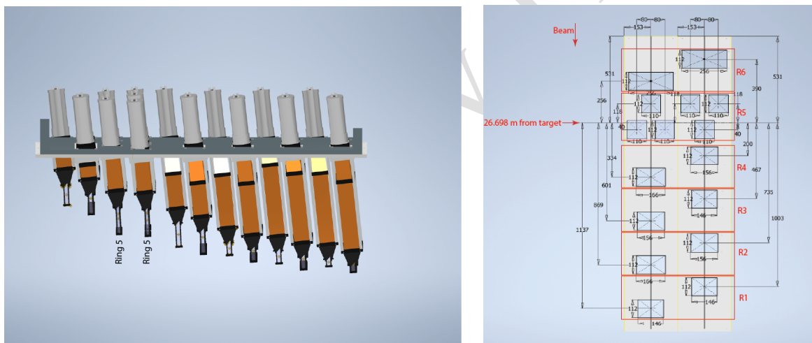
Figure 90: Left: CAD illustration of two adjacent front-flush and back-flush detector segments, illustrating the detector module positioning in the beam direction ( z -axis), with the beam travelling from left to right in the figure. Right: Front-flush and back-flush segment plates with module openings, illustrating the arrangement of the staggered detector elements.
