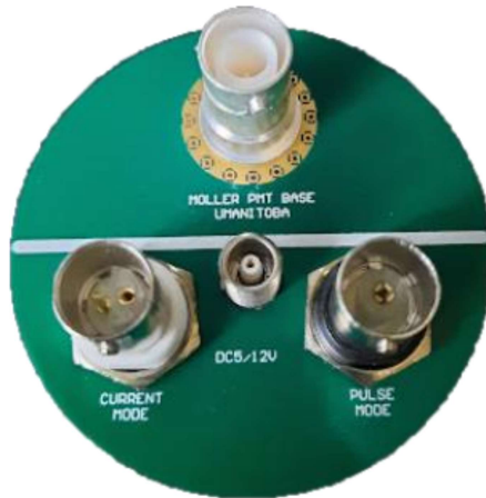
End-plate showing the layout of signal and power connectors
