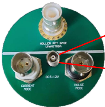
End-plate layout of scheme B & C
