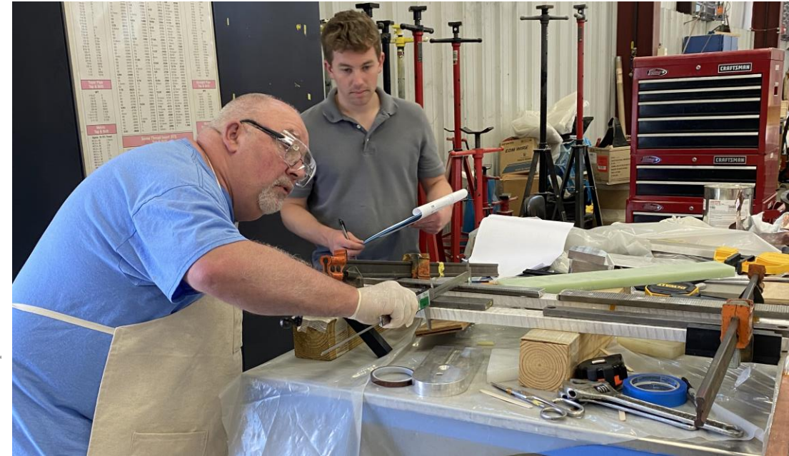
SC3 Post Winding Bending setup with ETI folks performing it
