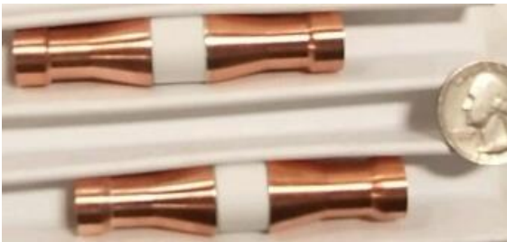
Ceramic break passed 1500psig hydro test
