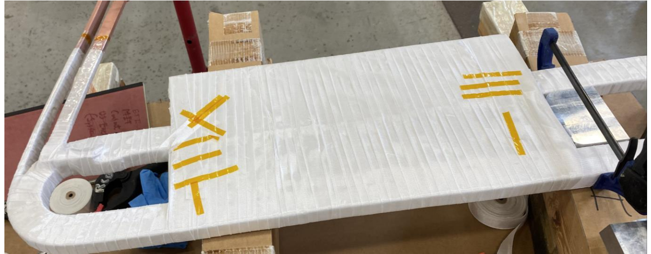
SC2 with Ground wrap – Did not fit in Mold
