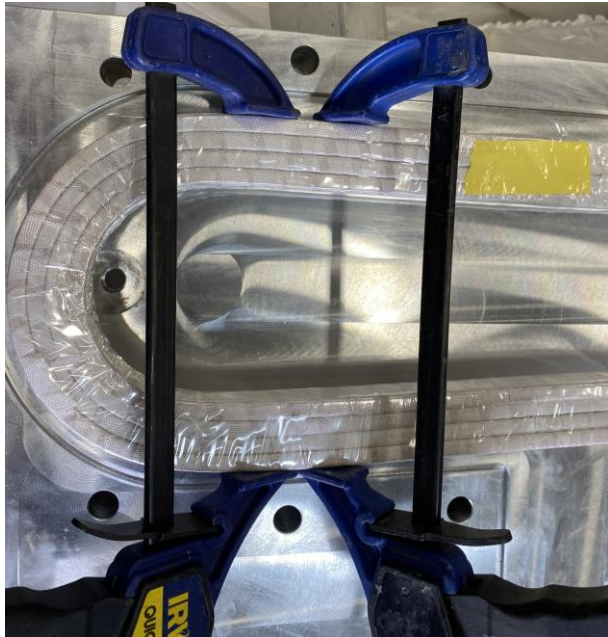
SC1 w/o Ground wrap – bending to attempt fit
