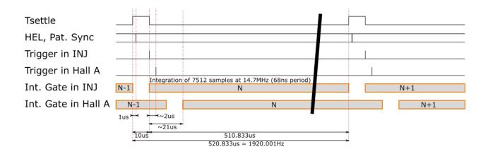
The helicity events are expected to be run at about 1920 Hz. A period of 520.833 us would permit the planned 10 us T\_settle and a 510.833 us stable helicity state.
