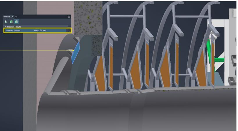
Lightguide should be long enough to tuck the PMTs inside the barite
