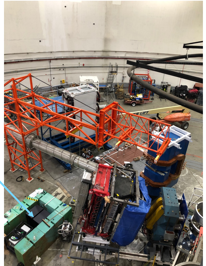
Small forward bunker for GEM electronics (MPDs) MOLLER may need one on each side of beamline
