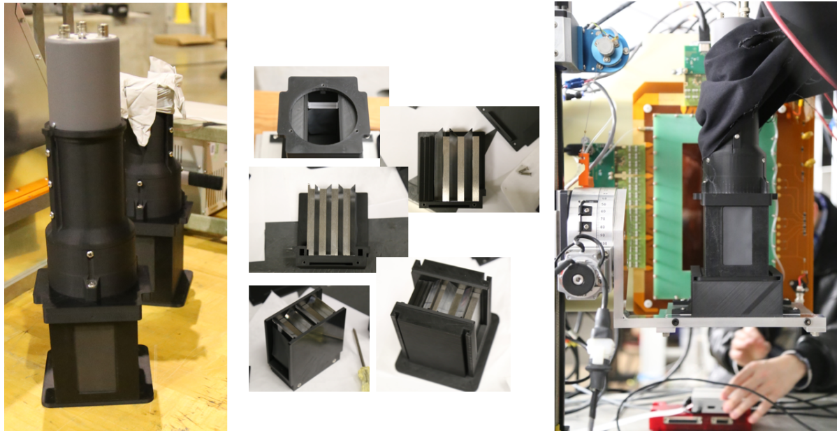
Figure 152: Benchmarking prototypes: (Left) Fully assembled 1A and 1B detectors. (Middle) Collage of photos during the stack assembly: shows views of the single quartz (top) as well as the 3- and 4-layer stack variations. (Right) Photo of the benchmarking prototype mounted in the SLAC testbeam stand.
